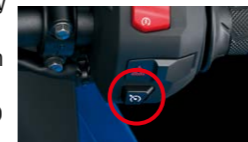
Cruise control system switch
